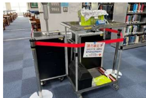
Regular indoor air quality inspection (CO 2 , PM 10 , formaldehyde) - Reading area of the Western-language book stacks on the 3rd floor of the library at the First Campus
