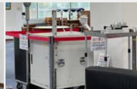
▲ Indoor air quality periodic inspection (CO 2 , PM 10 , Formaldehyde) at Current Periodicals Area, 2nd floor, Library and Information Center, First Campus
