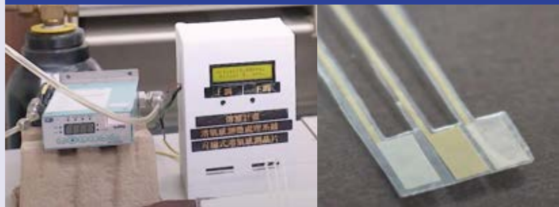
Development of a Disposable Chip-Based Dissolved Oxygen Sensing System for Live Fish Transportation
