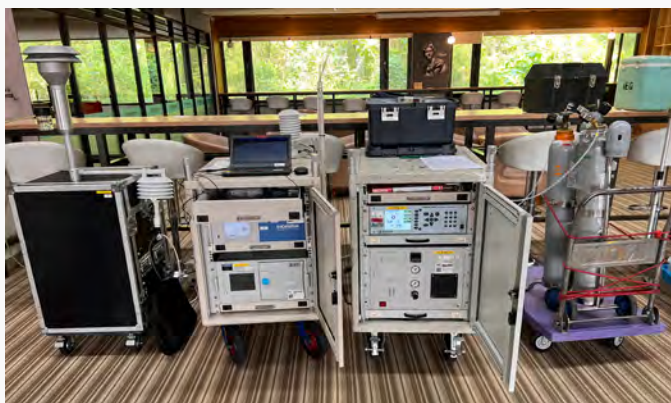
◀ Indoor air quality periodic inspection (CO 2 , PM10, Formaldehyde) at the Leisure Reading Area, 2nd floor, Yanchao Campus Library
